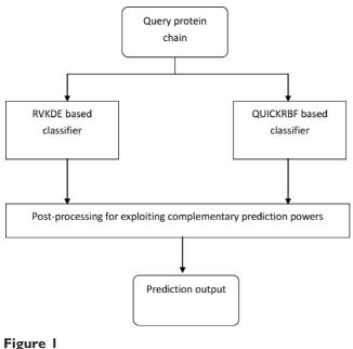
The overall structure of the proposed hybrid predictor.
