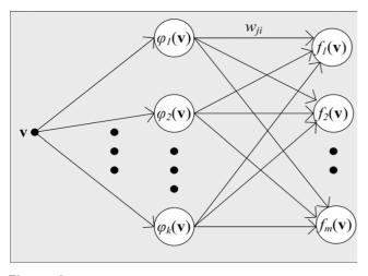
Figure 4 The schematic diagram of a RBF network.
